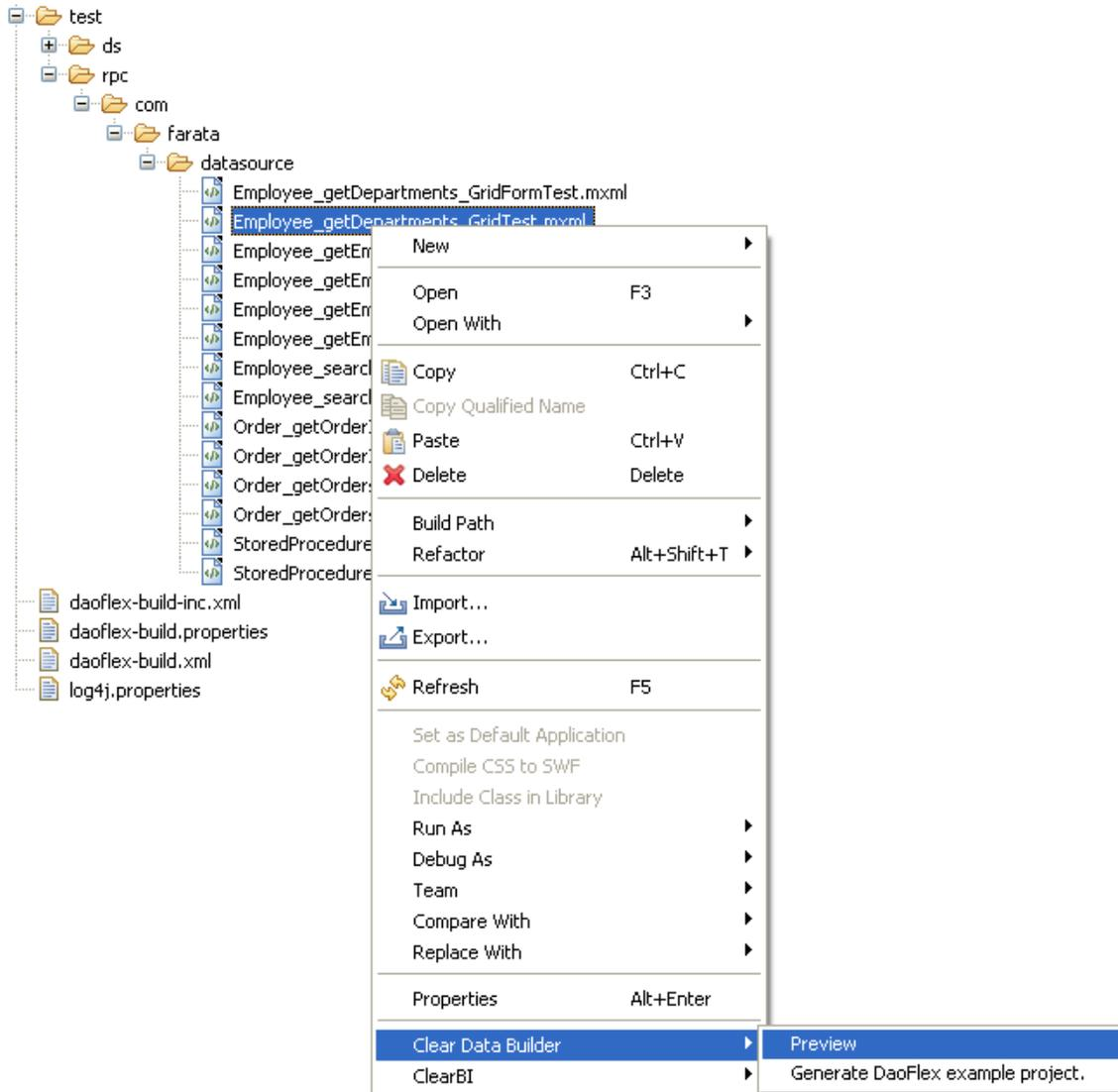
3. Clear Data Builder will compile the MXML file and will start created SWF in a special view Clear Data Builder SWF.
