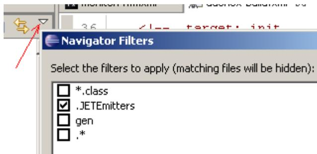
The generated Java code is located under the folder .daoflex-temp\gen. Re-run the Ant script to regenerate the code. If you do not see this folder immediately, refresh your Eclipse project by pressing F5.
