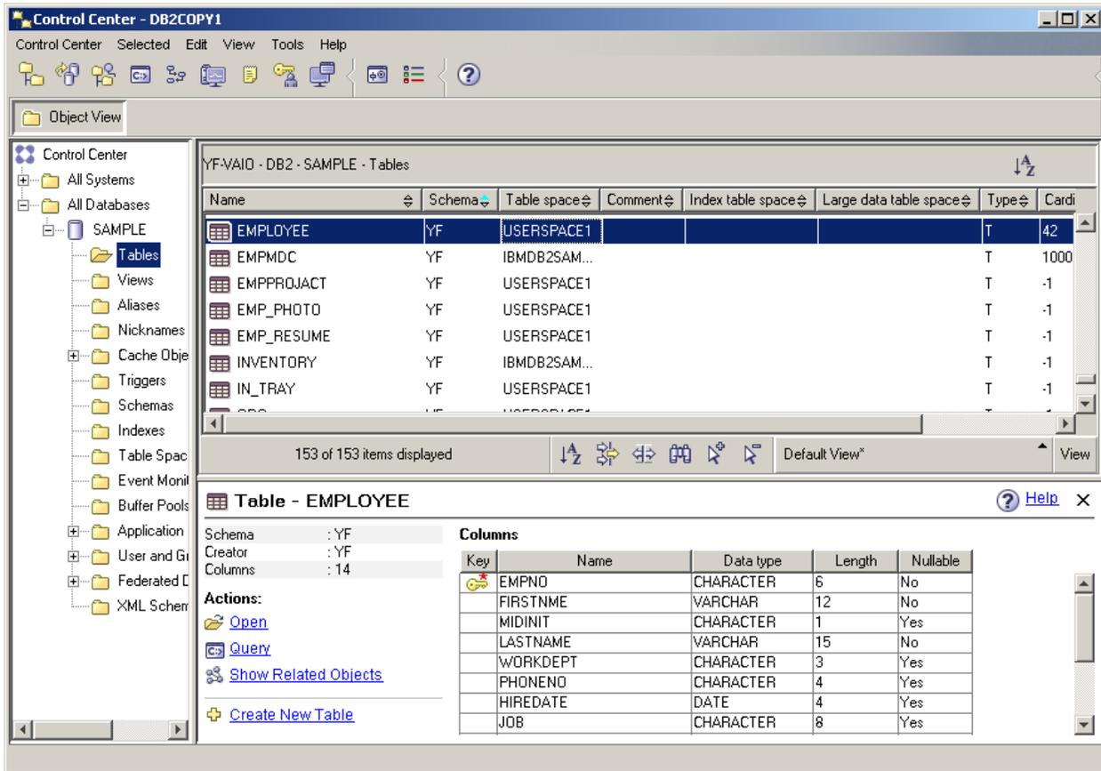
Since we configure the database connection pool using dba as a user id, we'd need to fully qualify the table name: `select * from yf.employee`. Accordingly, the name of the table to update should be also fully qualified.
